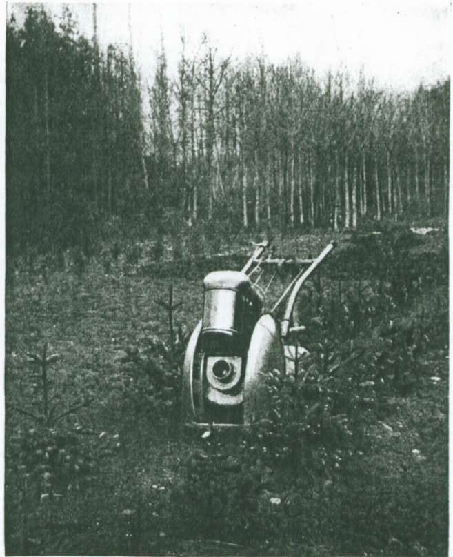
FIG. 21.—SIMAR ROTOTILLER 5 FIXED WITH SPECIAL WHEEL PROTECTIONS AS DESCRIBED ON PAGE 14.
